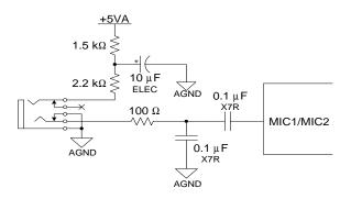
Figure 13. Microphone Input
