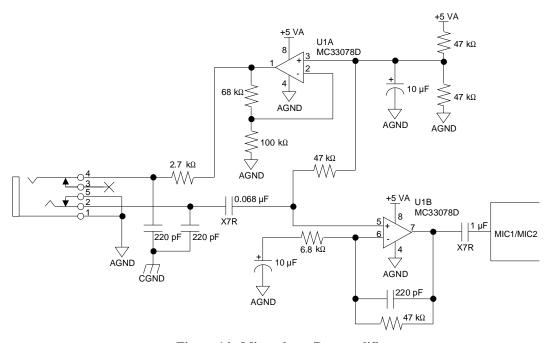
Figure 14. Microphone Pre-amplifier
