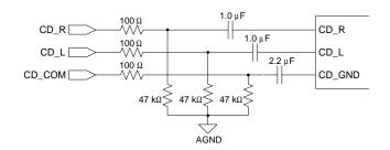
Figure 12. Differential 1 V<sub>RMS</sub> CD Input
