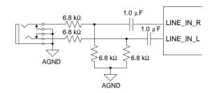
Figure 10. Line Input (Replicate for Video and Aux)
