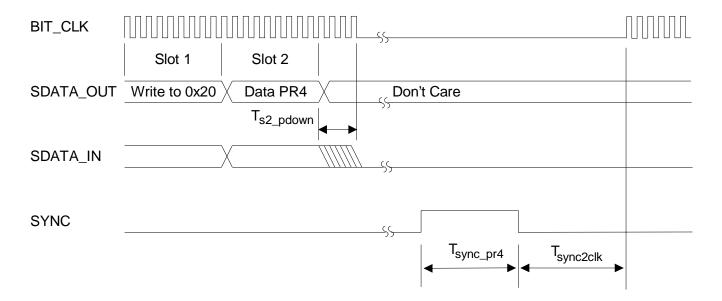
Figure 5. PR4 Powerdown and Warm Reset
