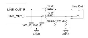
Figure 18. Stereo Output
