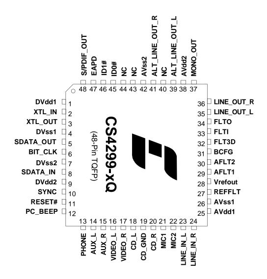
Figure 22. Pin Locations for the CS4299
