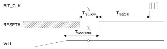
Figure 1. Power Up Timing
