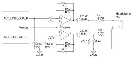
Figure 17. Alternate Line Output as Headphone Output
