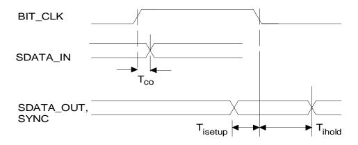
Figure 4. Data Setup and Hold
