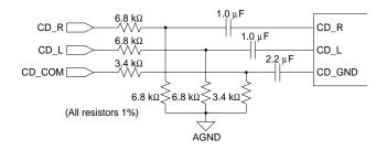
Figure 11. Differential 2  $V_{RMS}$  CD Input
