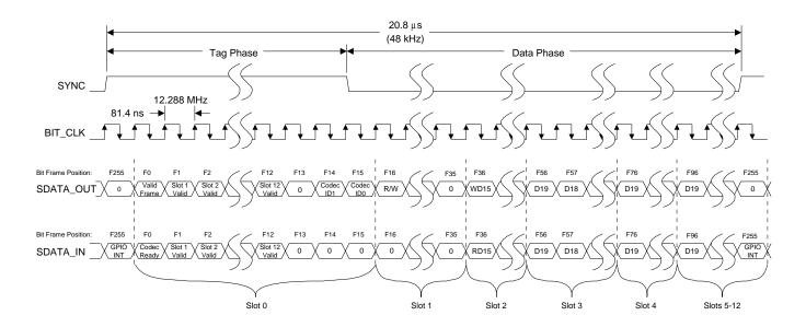
Figure 9. AC-link Input and Output Framing
