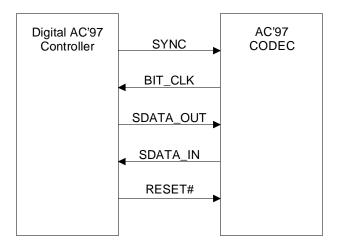
Figure 7. AC-link Connections
