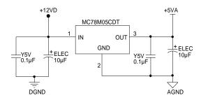
Figure 26. +5V Analog Voltage Regulator
