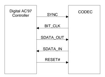
Figure 7. AC-link Connections
