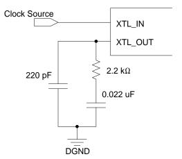
Figure 16. PLL External Loop Filter
