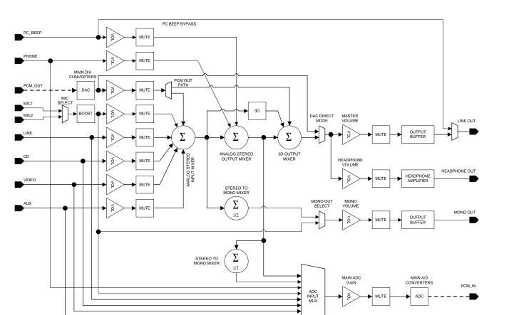
Figure 8. CS4201 Mixer Diagram
