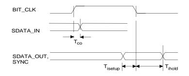
Figure 4. Data Setup and Hold
