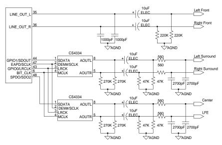
Figure 10. Serial Data Port: Six Channel Circuit
