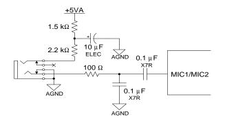
Figure 21. Microphone Input
