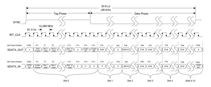
Figure 9. AC-link Input and Output Framing
