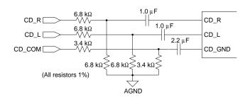
Figure 19. Differential 2  $V_{RMS}\ CD$  Input
