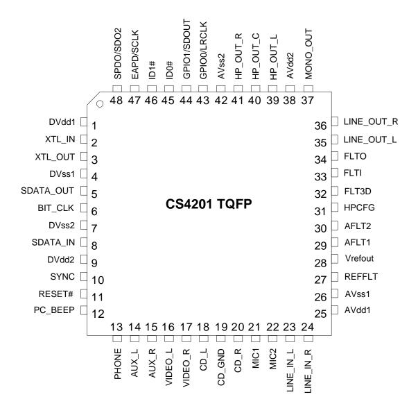
Figure 28. Pin Locations for the CS4201
