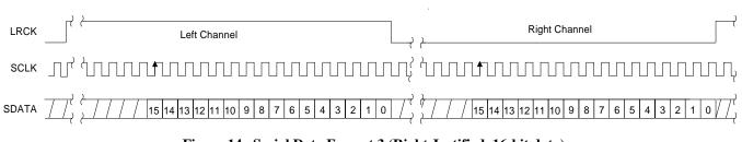
Figure 14. Serial Data Format 3 (Right Justified, 16-bit data)
