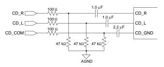
Figure 20. Differential 1  $V_{RMS}$  CD Input
