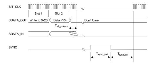
Figure 5. PR4 Powerdown and Warm Reset
