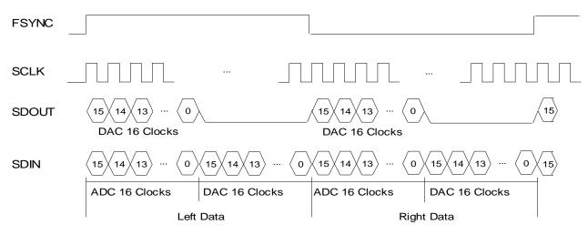
Figure 13. Serial Audio Port Format for CS4610/11 + CS423XB Configuration
