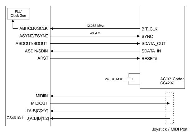
Figure 16. CS4610/11 - AC '97 Codec Connection Diagram
