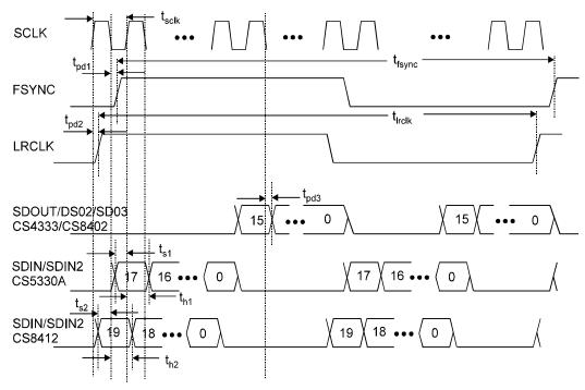
Figure 5. Independent Timing Configuration
