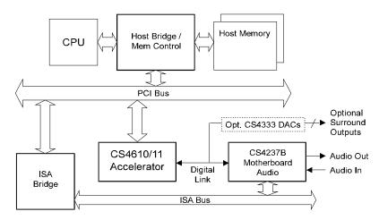
Figure 9. CS4610/11 + CS423XB Motherboard Audio Configuration
