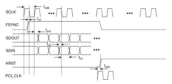
Figure 4. AC97 Configuration Timing Diagram
