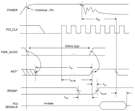
Figure 2. Reset Timing
