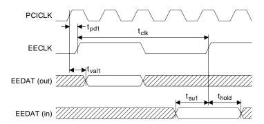
Figure 6. EEPROM Timing Characteristics
