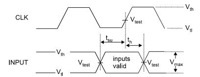
Figure 7. Input Timing Measurement Conditions
