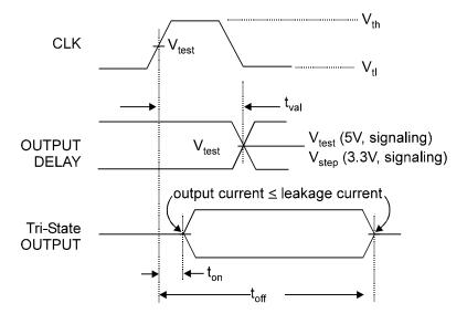
**Figure 8. Output Timing Measurement Conditions**
