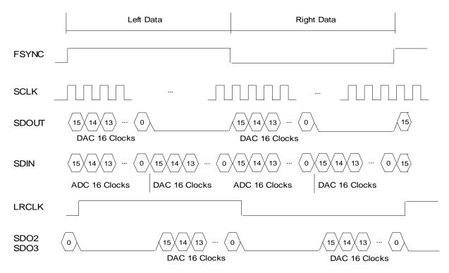
Figure 15. Serial Audio Port Format for CS4610 + CS423XB Expanded Output Configuration.
