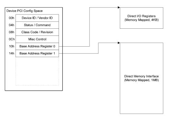
Figure 11. CS4610/11 Host Interface Base Address Registers
