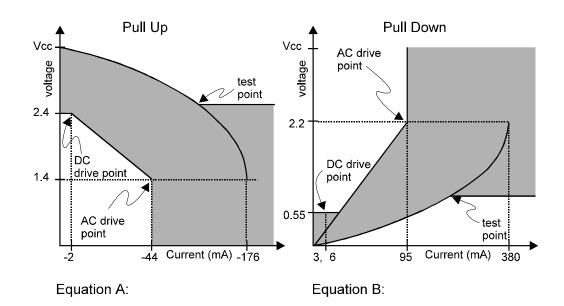
Figure 1. AC Characteristics
