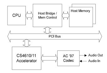
Figure 10. CS4610/11 + AC '97 Codec Configuration
