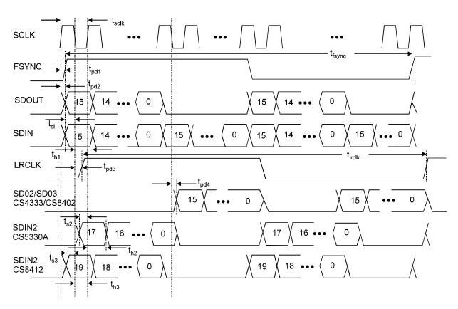
Figure 3. CS4610/11 and CS423XB Link and AC3 Expanded Timing Diagram
