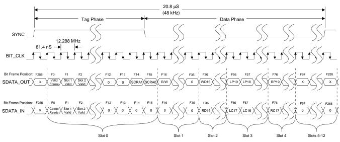
Figure 2. AC-link Input and Output Framing
