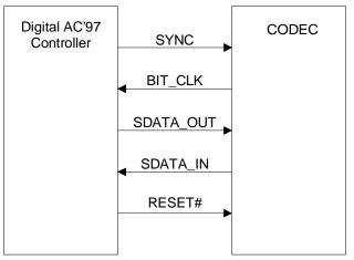
Figure 1. AC-link Connections
