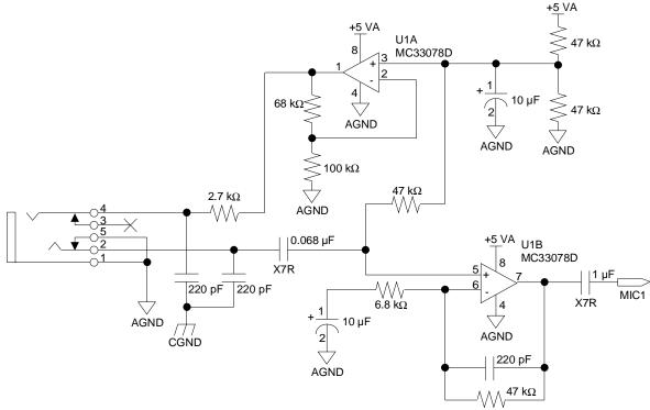
Figure 6. PC '99 Microphone Pre-amplifier
