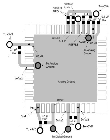
Figure 11. Suggested Layout for the CS4297A
