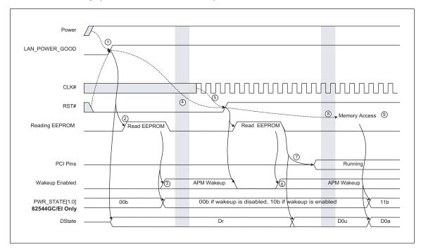
Figure 6-2. Startup Timing
