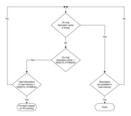
Figure 3-1. Receive Descriptor Fetching Algorithm
