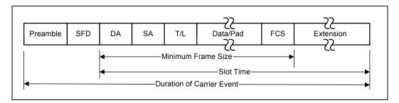
Figure 13-1. Carrier Extended Frame Format (82541xx and 82547GI/EI)
