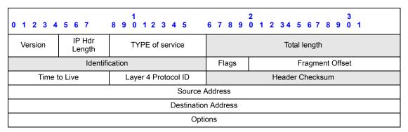
Figure 3-8. IPv4 Header (Traditional Representation)
