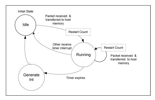
Figure 3-3. Packet Delay Timer Operation (State Diagram)
