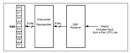
Figure 11-5. 1000BASE-T Receive Flow
