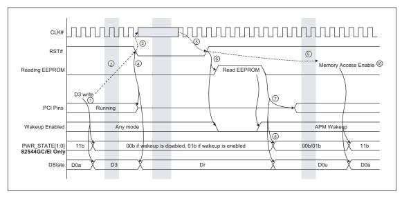
Figure 6-4. Transition From D0a to D3 and Back with PCI Reset
