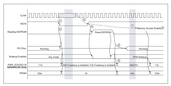
Figure 6-5. PCI Reset Sequence
