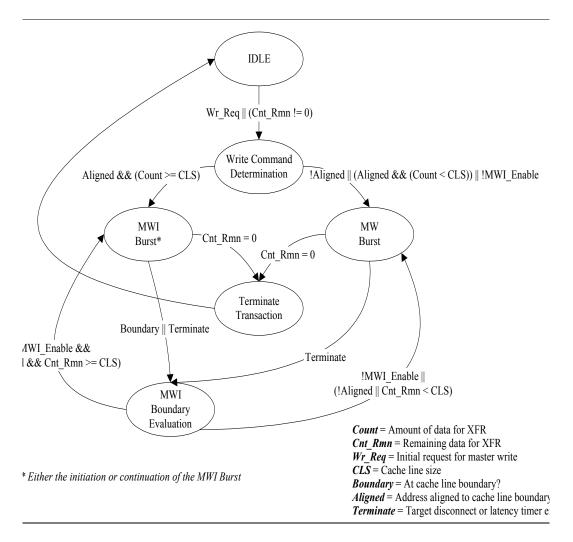
Figure 4-4. Master Write Command Usage Algorithm
