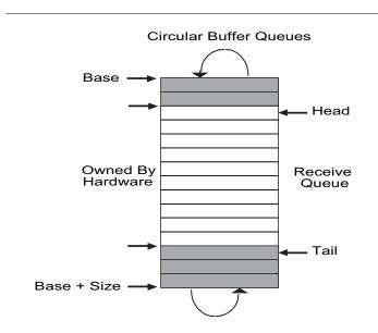
Figure 3-2. Receive Descriptor Ring Structure
