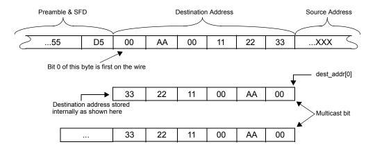
Figure 2-5. Example of Address Byte Ordering
