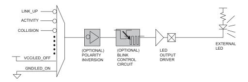
Figure 10-1. Selecting an LED Output Source
