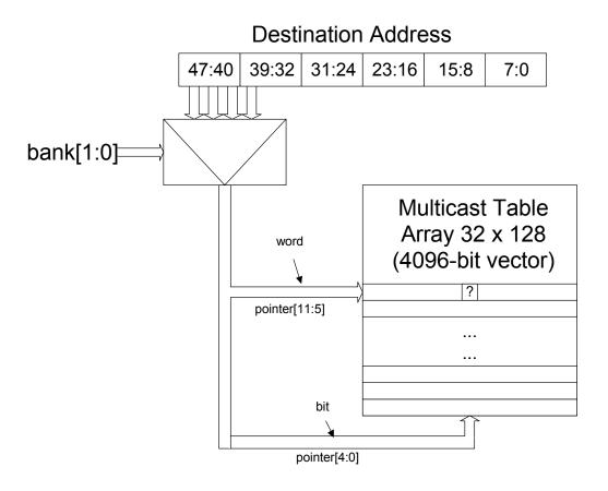
Figure 13-2. Multicast Table Array
