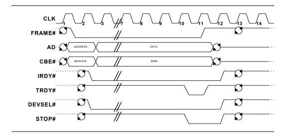
Figure 7-2. FLASH Buffer Write Cycle
