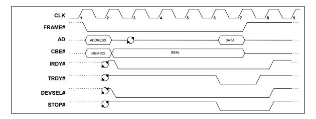
Figure 7-1. FLASH Buffer Read Cycles
