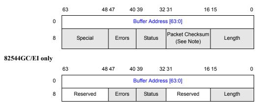
**Note:** The checksum indicated here is the unadjusted "16 bit ones complement" of the packet. A software assist may be required to back out appropriate information prior to sending it to upper software
