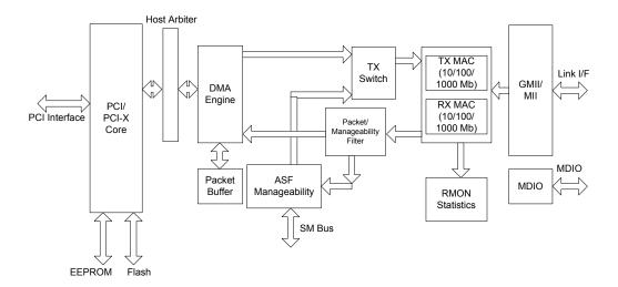
Figure 2-4. Internal Architecture Block Diagram
