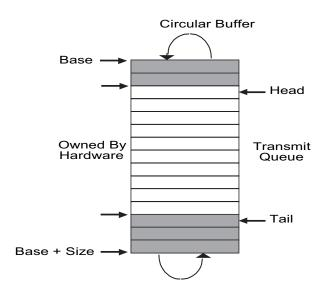
Figure 3-4. Transmit Descriptor Ring Structure
