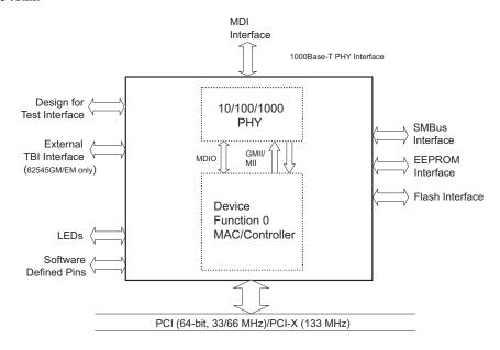
Note: 82540EP/EM and 82541xx do not support PCI-X; 82544GC/EI and 82541ER do not support SMBus interface
