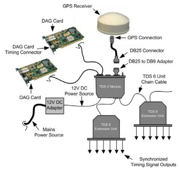
TDS2 modules and TDS6 units require 12VDC either via an adapter connected to a mains power supply or directly from a 12VDC source.
