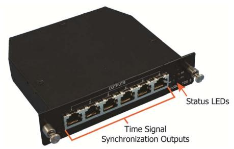
A TDS6 Expansion unit connects to the Chain output on the TDS2 Server Module. The synchronized time signals travel from the TDS2 Chain port to TDS6 expansion units through chain cables. The signals travel to DAG cards via the TDS6 Expansion unit synchronization outputs.
